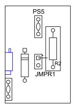
**ASIC/1-6000 or ASIC/1-8x00:** Move jumper JMPR1 to the closed position.
